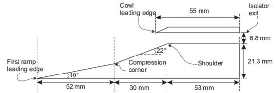
Figure 2: Generic scramjet inlet and its dimensions<sup>6</sup>
