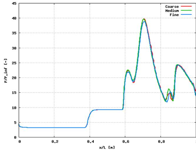
Figure 5: The comparison of different grid refinement levels
