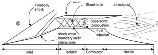
Figure 1: Generic diagram of a scramjet engine<sup>6</sup>
