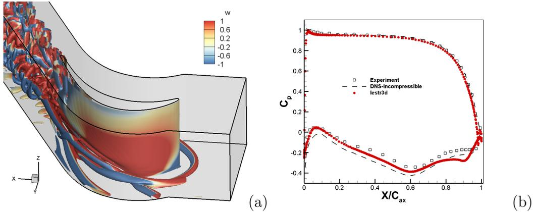
**Figure 2:** Q criterion isosurfaces coloured by the spanwise velocity fluctuations (a). Pressure coefficient distribution on blade surface at  $z/h = 0.5$ , compared with experiment and DNS results [11] (b).
