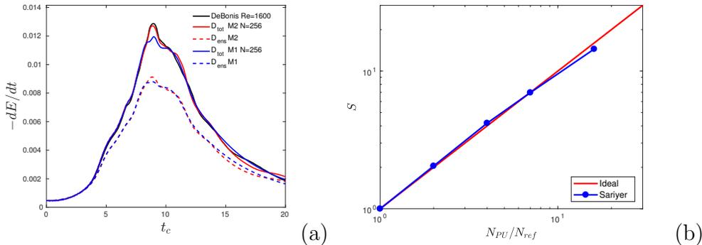
**Figure 1:** Change of kinetic energy dissipation (solid) and entropy related dissipation  $D_{ens}$  (dashed) with convective time  $t_c = L/V_0$  compared with results from DeBonis [10] (a) Speed-up of the code (b).
