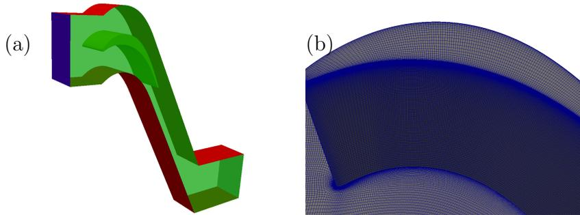
Figure 1: Computational domain (a) with periodic surfaces (red), tip end wall (green), inlet (blue) and close view to the grid map around the blade surface (b).
