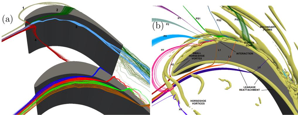
Figure 3: Visualization of blockage of the upstream flow (a) and coherent structures with relevant streamlines (b).
