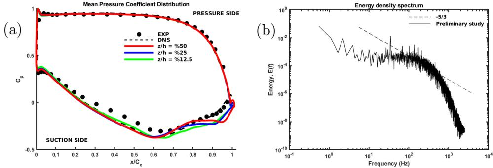
Figure 2: Time-averaged mean pressure coefficient at three cross-sections compared with DNS and experimental results (a) [8], energy density spectrum (b).
