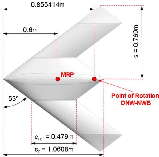
Figure 1: SACCON Reference Values and Geometry
