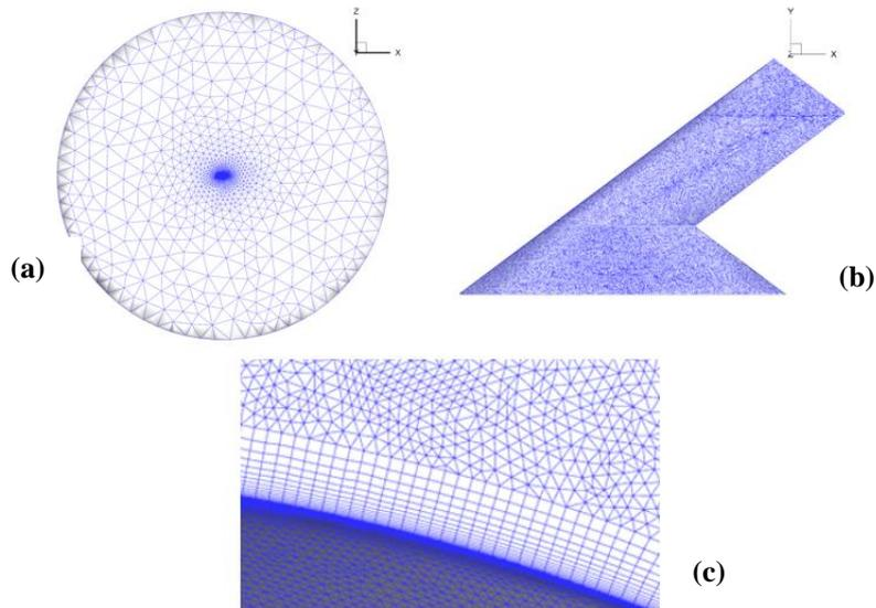
Figure 3: Computational grid around SACCON model (a) Overall grid, (b) Surface grid on right-half of the model, (c) Boundary layer grid
